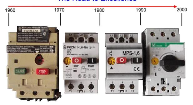
The older style PKZM0-xx-NA was replaced by the PKZM1 series. The PKZM1 series was temporarily replaced with the MPS series. The older styles ( PKZM0-xx-NA, PKZM1-xx, MPS-xx ) are now retired and replaced with the upgraded PKZM0 series. The PKZM1 & MPS are identical in form, fit, function and rating's, however the modern updated series PKZM0 is quite different and upgraded.
